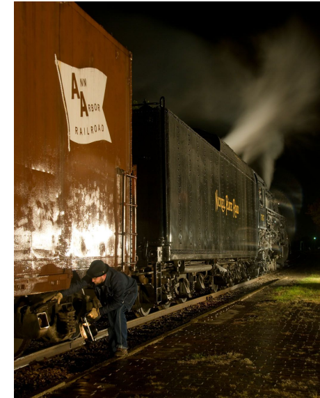
Scene 4: Crew member checking bearing boxes with locomotive in the background.
